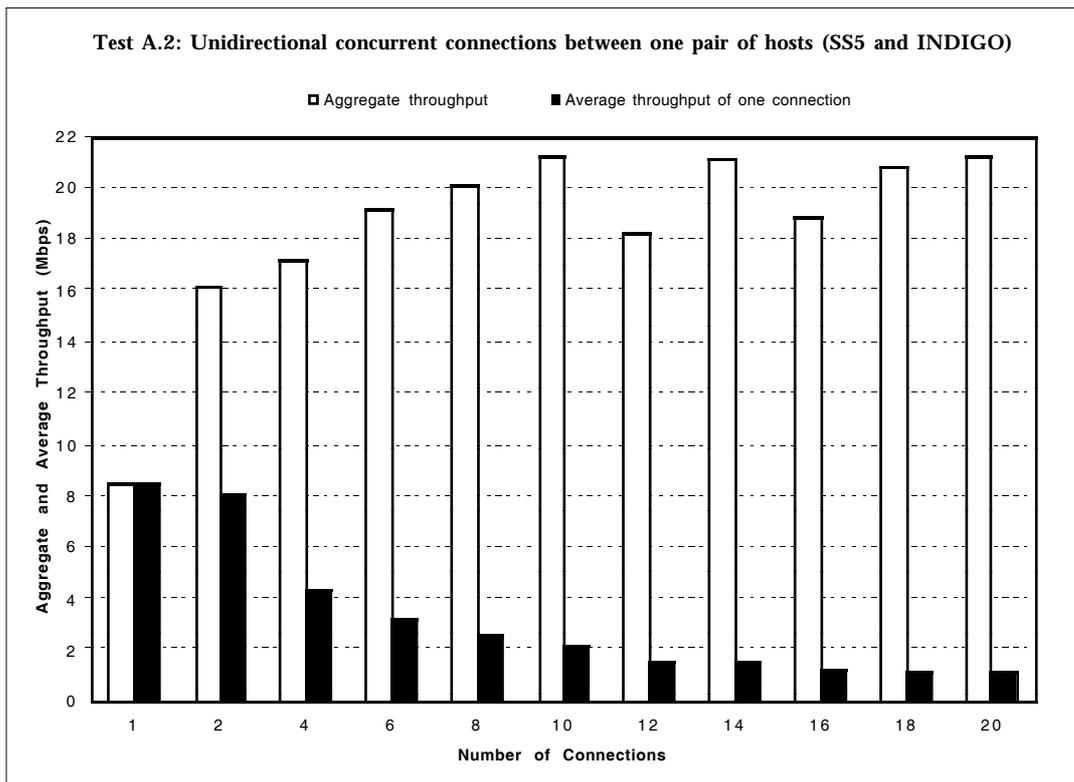
Figure 6: Test session Italy-Sweden: Aggregated throughput for a bunch of one-way TCP connections between 1 pair of end-nodes.
