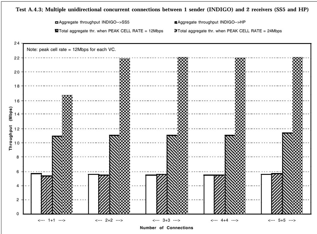
Figure 12: Comparison of aggregated throughputs achieved for 2 distinct bunches of one-way TCP connections from 1 sender to 2 receivers with different peak cell rate configurations.
