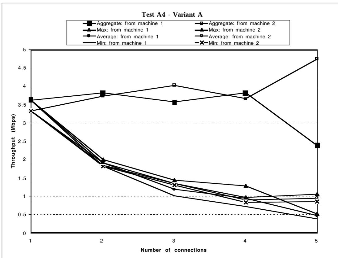
Figure 9: Test session Norway-Spain: aggregate throughput for 2 bunches of TCP connections from 2 senders to 1 receiver and with PCR = b on each VC.
