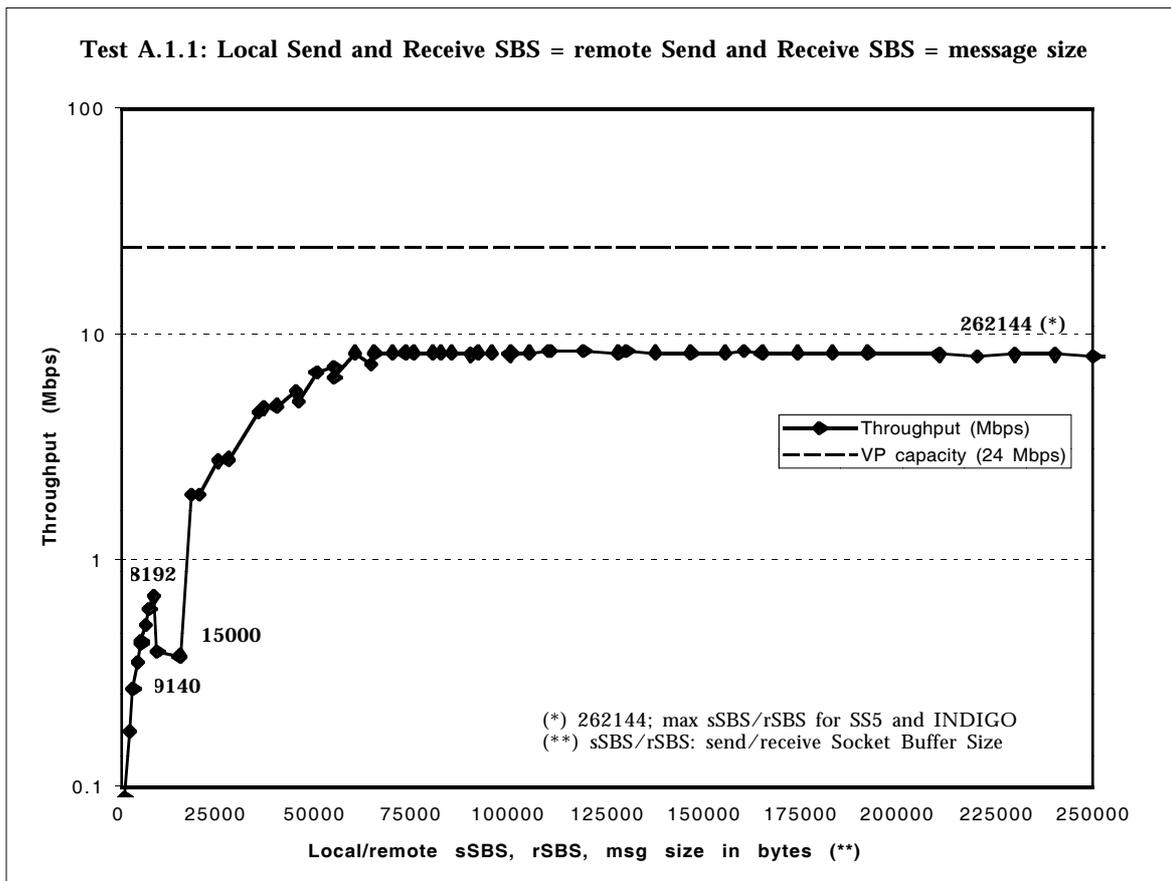
Figure 4: Test session Italy-Sweden: Throughput measurement for a one-way TCP connection with variable local ssb/rsb sizes ,remote ssb/rsb sizes and message size (ssb = rsb = msg).
