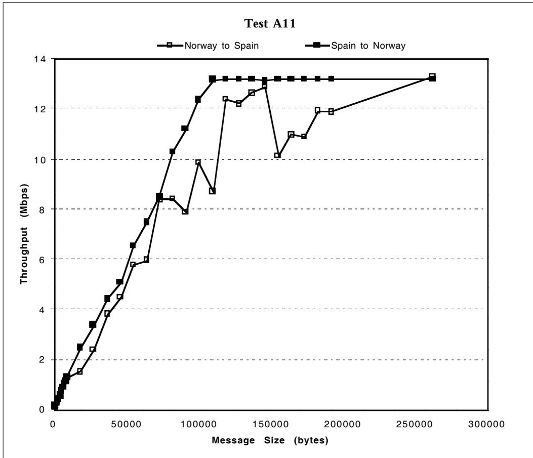
Figure 3: Test session Norway-Spain: Throughput measurement for a one-way TCP connection with variable local *ssb/rsb* sizes, remote *ssb/rsb* sizes and message size (*ssb = rsb = msg*).
