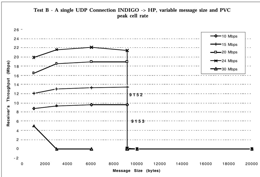
Figure 11: Relationship between variable peak cell rate (PCR) configured for the ATM VC and throughput achieved by a single one-way TCP connection on top of the VC itself.
