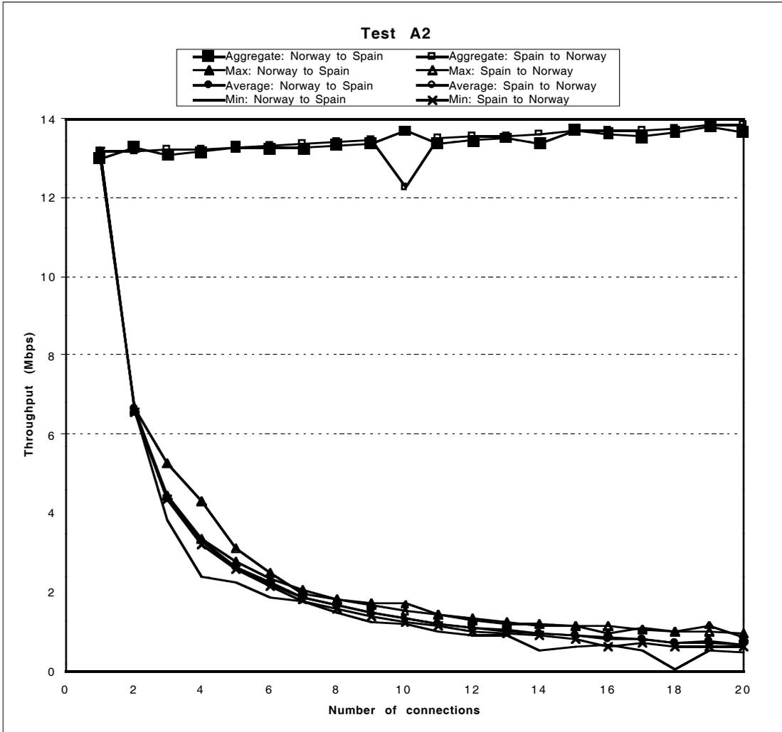
Figure 5: Test session Norway-Spain: Aggregated throughput for a bunch of one-way TCP connections between 1 pair of end-nodes.
