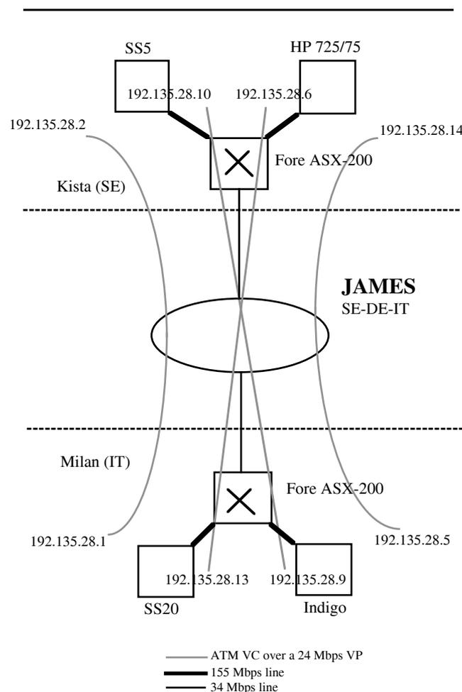
Figure 1: Equipment and network configuration in the test session Italy-Sweden.
