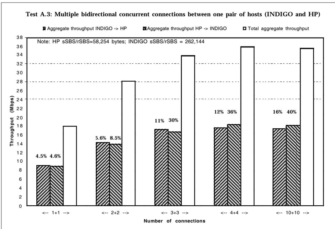
Figure 8: Test session Italy-Sweden: Test of aggregate throughput for a bunch of two-way TCP connections between two end-nodes.
