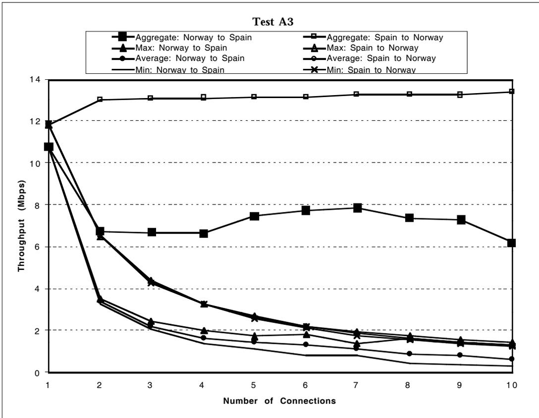
Figure 7: Test session Norway-Spain: Test of aggregate throughput for a bunch of two-way TCP connections between two end-nodes.
