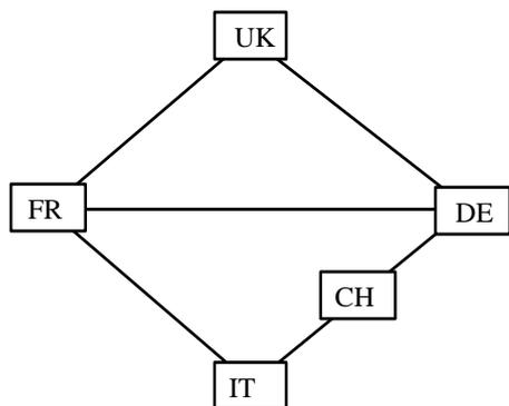
figure 1: Planned FUDI topology; the boxes are ATM switches.
