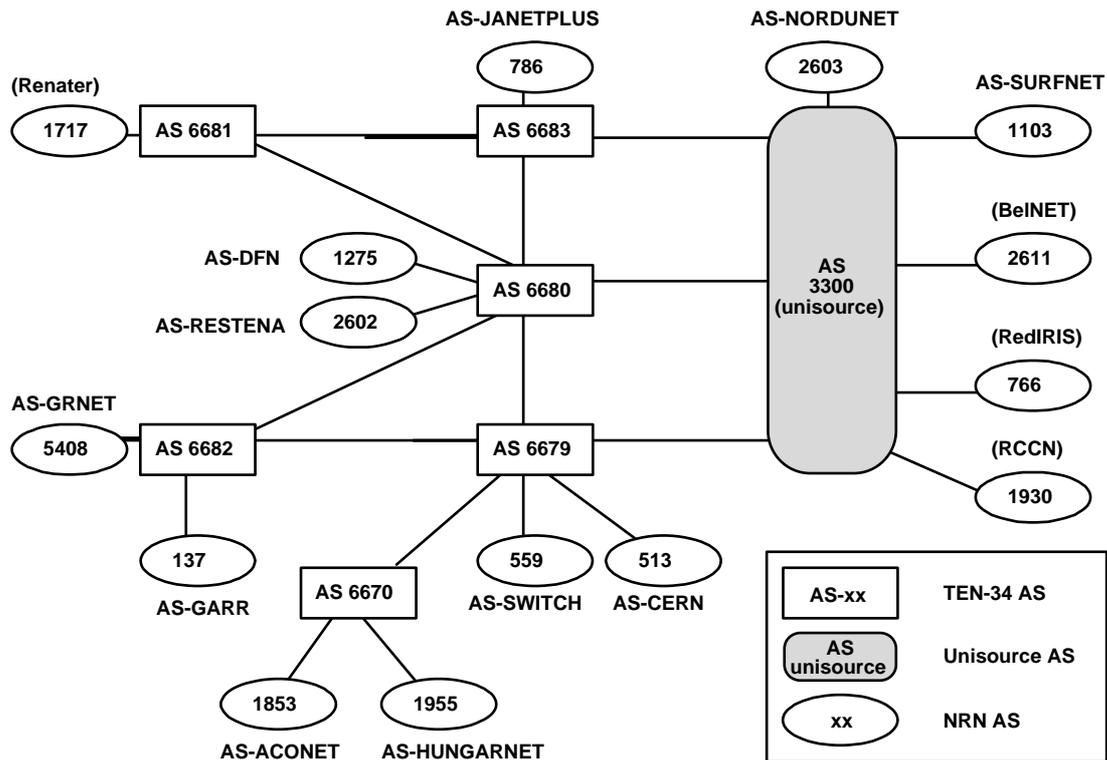
Figure 2: TEN-34 routing set-up.
