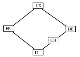
figure 1: Planned FUDI topology; the boxes are ATM switches.
