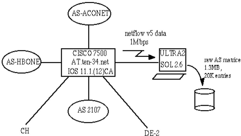
Figure 1.1 illustrates an example PoP set-up. Netflow is enabled on all of the TEN-34 router's interfaces. The netflow data is exported to the locally connected workstation. The amount of traffic generated by netflow is proportional to the amount of traffic that flows through the router.
