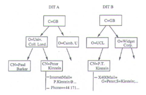
Figure 3: Parallel and over-lapping DITs
