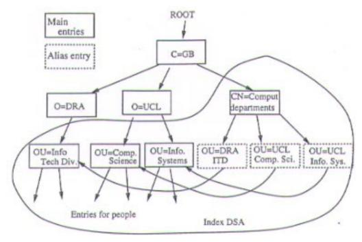
Figure 6: Computer personnel data replicated into Index DSA
