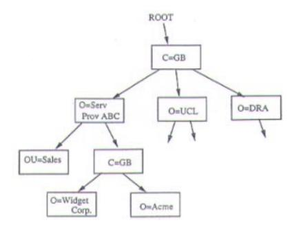
Figure 4: Additional Organisation Entries Beneath Service Provider Entry
