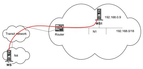
Figure 5. Forged IP addresses within prefix range of machines
