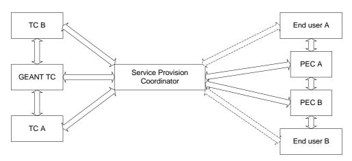
Figure 2.4-3. Parties involved in the provisioning of Premium IP service
