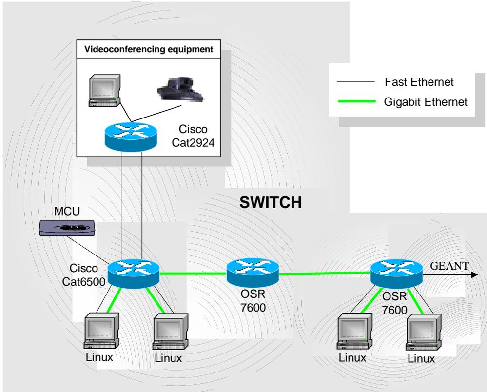
**Fig. 9. SWITCH test case topology.**
