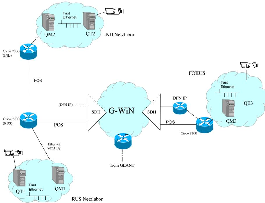
**Fig. 7. Quasar network detailed topology for H323 tests.**
