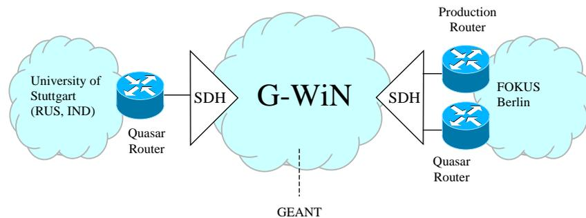
**Fig. 6. Topology of the Quasar testbed for H323 tests.**
