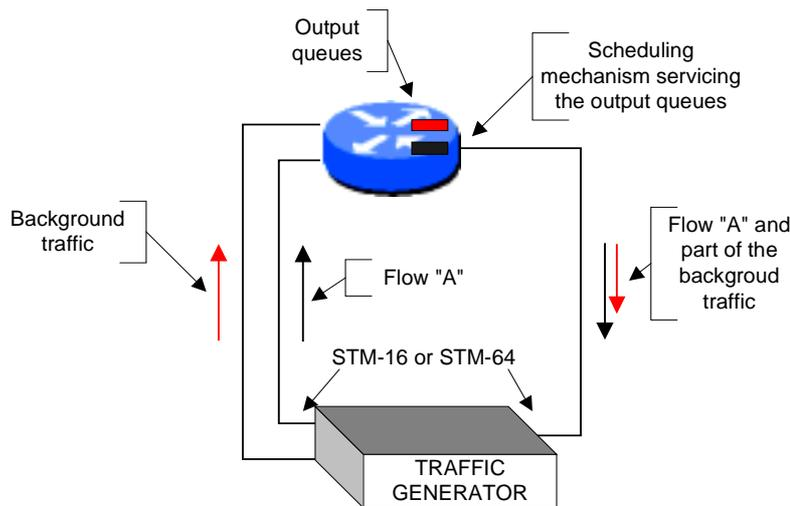
**Fig. 2. Test of Scheduling mechanisms.**
