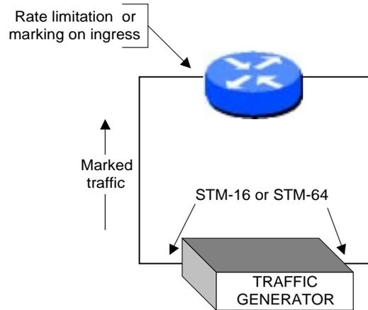
**Fig. 1. Topology of the first rate limitation test.**
