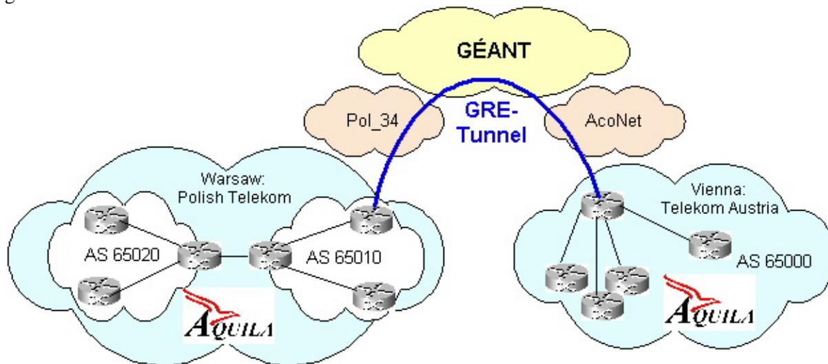
**Figure 3.2-1: AQUILA testbed description**
